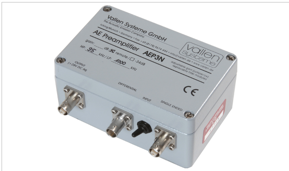
Figure 2: AEP3N preamplifier. Connectors from left to right are: (i) signal output and power supply input, (ii) differential BNC input and (iii) single ended BNC input.
